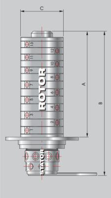
Stainless Steel Fluid / Gas Swivel for Offshore Winches
